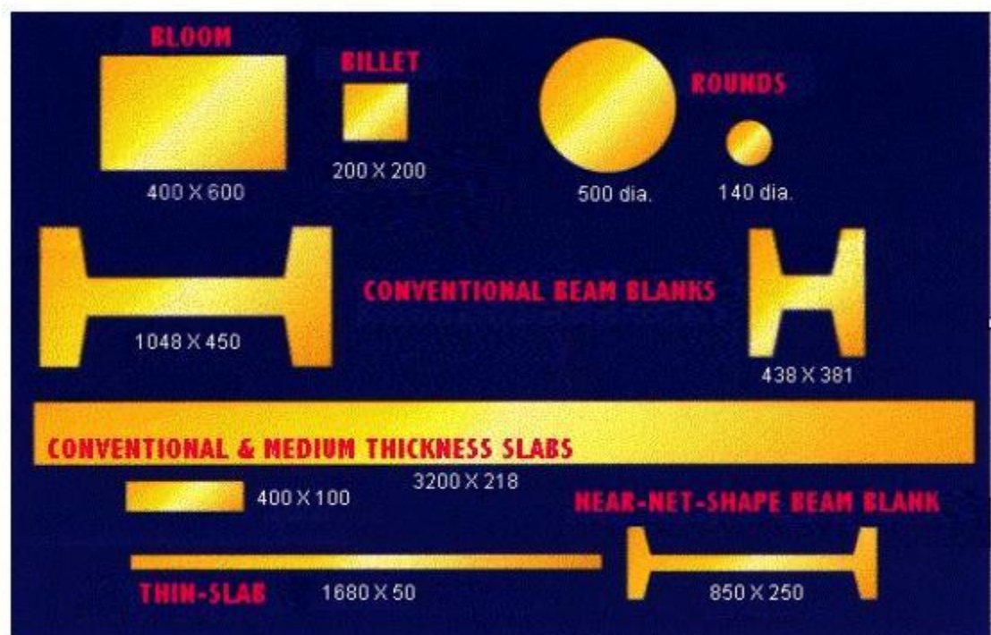
Figure 4 - Continuous Cast Shapes (sizes in millimeters)
