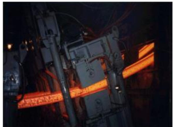
Figure 8 - Straightener Withdrawal Units for Strand Unbending
